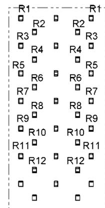
Recommended PCB Layout. Component side of board
